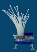
The Chimera innovates the analysis process by automatically reading CH<sub>4</sub> and CO<sub>2</sub> composition online, from a maximum of 15 individual reactors. It only requires a gas sample of 15ml, allowing for more frequent and holistic analysis, as well as maintaining functionality under low gas flow conditions such as standard BMP tests.
