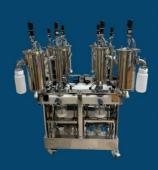
Boasting many possible configurations, the Black Swan is our most comprehensive multi-stage model. With four 1st stage and four 2nd stage reactors (+optional additional stages), and 4 auto-feeders, the Black Swan allows you to compartmentalise the AD process by configuring each stage through temperature control and HRT.
